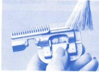
Figure 7 — Separate the cutting edges of the blade as shown and brush away any loose matter. Hold the blade to the light to make sure that no small hairs are caught in the teeth.
