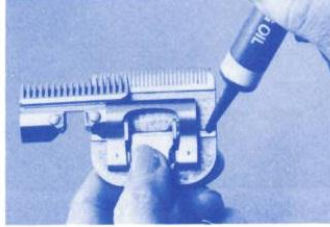
Figure 4 — Be sure to place one drop of oil on each running rail.
