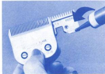
Figure 5 — Remember, do not drop oil on the teeth of your blade, only on the running rails.
