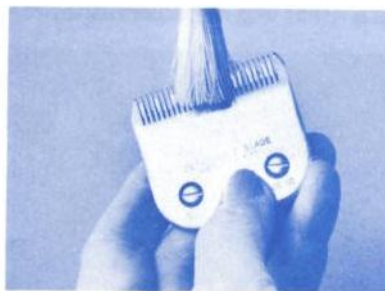
Figure 6 — Use the brush provided with your clipper kit to remove hair and debris from between the blade teeth. If it has been lost or worn out, use an old toothbrush, or vegetable brush as shown here.
