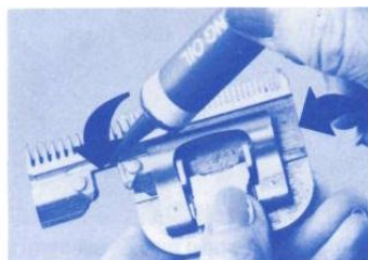
Figure 3 — After using Blade Wash, oil the running rails and use only a drop of oil.
